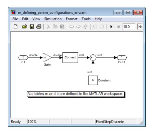
The PreLoadFcn callback function defines m and b in the MATLAB workspace when you open the model:
