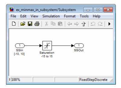
In Subsystem, the specified minimum and maximum values for input port SSIn are -10 and 10, respectively. The lower and upper limits for the Saturation block are -15 and 15, respectively.
