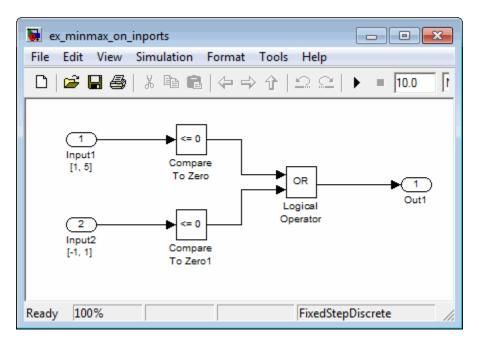
When you analyze this model using the Simulink Design Verifier software, the analysis uses the minimum and maximum values as constraints. The analysis produces the following results:
