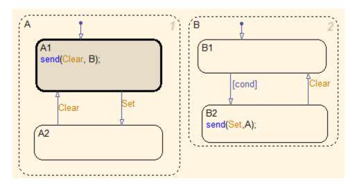
If you change the send function calls to use directed event broadcasts so that the Set and Clear events are broadcast directly to the states B1 and A1, respectively, the cyclic behavior disappears and the Simulink Design Verifier software can analyze the model.
