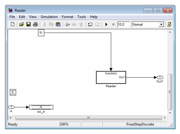
The new Inport block A writes into the data store, which is used by the subsystem Reader in the new model.
