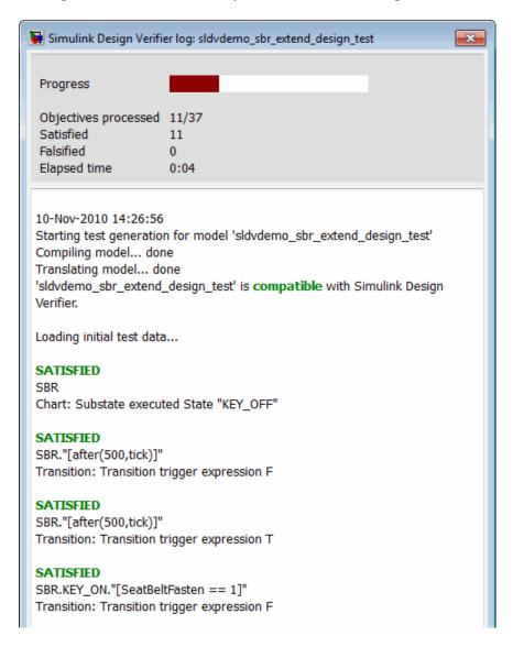
The log window then lists the objectives generated beyond the starting test case.
