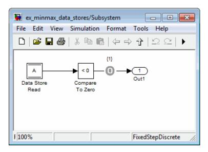
If you right-click Subsystem in the top-level model and select **Generate Tests for Subsystem**, the analysis considers the constraints for data store A to be [0, 10].
