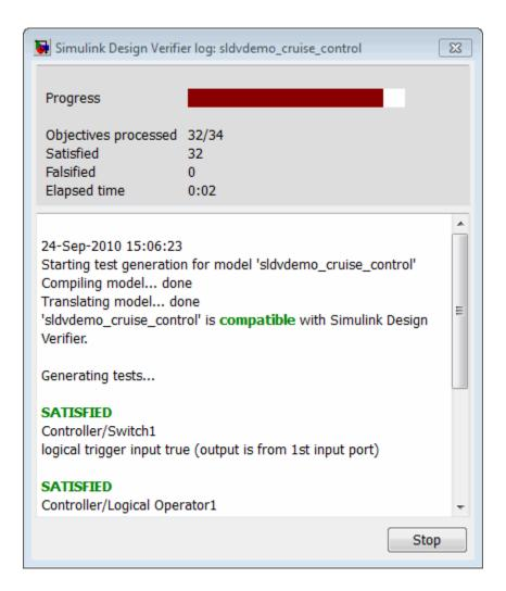
The log window shows you the progress of the Simulink Design Verifier analysis.
