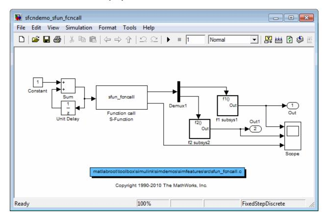
The Simulink Design Verifier software does not support the S-Function block, so if automatic stubbing is enabled, the analysis ignores the behavior of the S-function. As a result, the code that triggers the two function-call subsystems is ignored, resulting in two unsatisfiable objectives. Since the function calls are ignored, the contents of those subsystems are effectively eliminated from the analysis.
