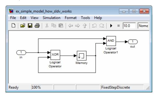
The persistent information in this model is limited to the Boolean value of the Memory block. The input to the model is a single Boolean value. The following table describes the complete behavior of the model, including the behavior that would result from an arbitrarily long sequence of inputs.
