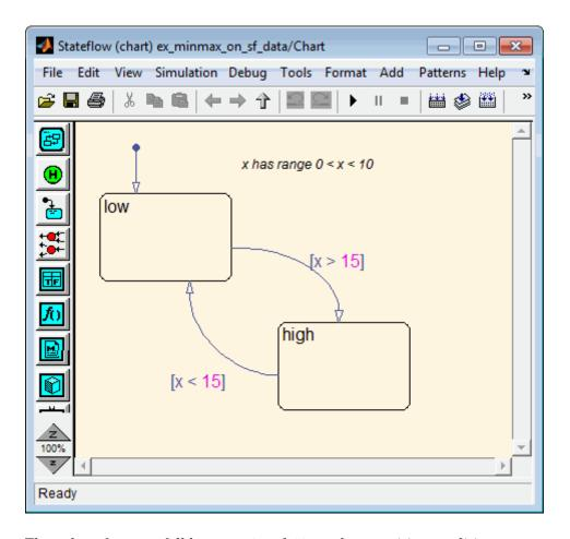
The value of x must fall between 0 and 10, so the transition condition [x > 15] is never true. The transition from low to high never occurs. Because the high state is never entered, the transition condition [x < 15] is never tested, and the transition from high to low never occurs; the chart is always in the low state.
