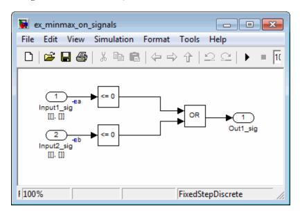
When you analyze this model, the results are the same as if you specified the minimum and maximum values on the input ports.
