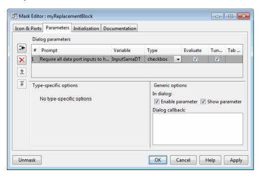
**Note** When you create mask parameters that control the behavior of parameters associated with their underlying blocks, specify actual parameter names as dialog box variables in the Mask Editor. For instance, InputSameDT is the actual parameter name that controls the Require all data port inputs to have the same data type parameter of the Multiport Switch block; therefore, it specifies the name of the dialog box variable in this example.
