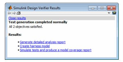
**Tip** By default, the Simulink Design Verifier Results window is always the topmost visible window. To allow the window to move behind other window, click **3** and clear **Always on top**.
