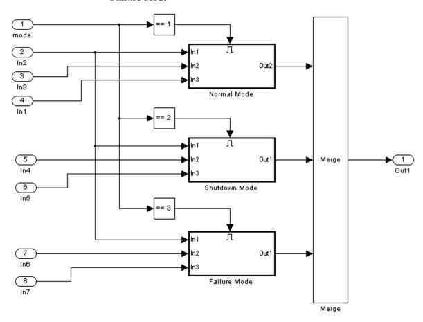
You can incrementally generate test cases for each subsystem by constraining the first input to a constant value before running an analysis. In this way, as you create test cases for each subsystem, the software ignores the complexity of the other two subsystems.
