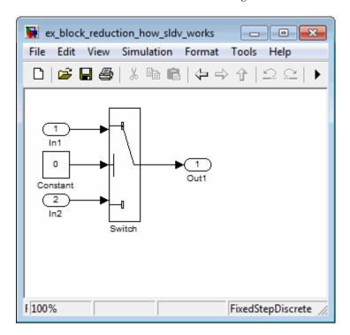
For this Switch block, the control input is always 0. If the **Criteria for passing first input** block parameter is u2 ~= 0, the Switch block always passes the third input through to the output port. When you analyze this
