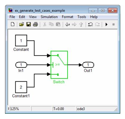
The Switch block is outlined in green, which indicates that the Switch block has test cases that satisfy its test objectives.
