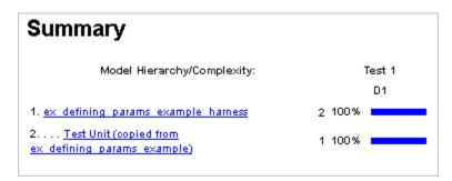
This section summarizes the coverage results for the harness model and its Test Unit subsystem. Observe that the subsystem achieves 100% decision coverage.
