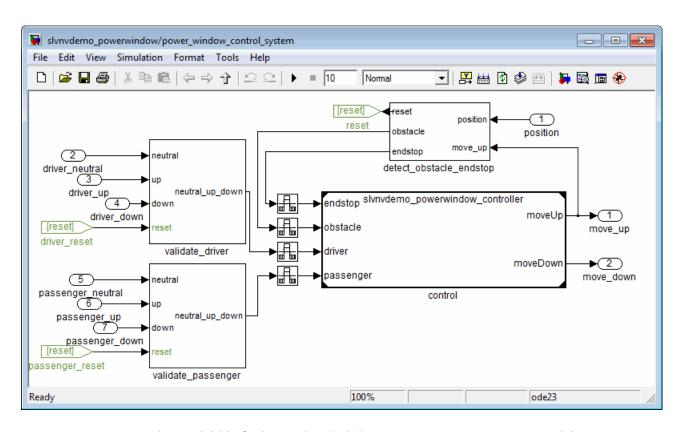
The Model block the top level of the  $slvnvdemo\_powerwindow$  model. references the  $slvnvdemo\_powerwindow\_controller$  model.
