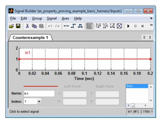
The input signal 1 causes the output of the Compare to Zero block to be 0. This counterexample violates the proof objective that specifies that the output of the Compare to Zero block be 1.
