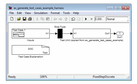
The Signal Builder block named Inputs contains the test cases. Double-click the Inputs block to see the test cases. From the Signal Builder block, you can simulate the model using the test cases and produce a model coverage report, as described in "Simulating Tests and Producing a Model Coverage Report" on page 7-16.
