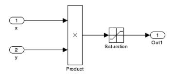
The Simulink Design Verifier software generates errors when attempting to satisfy the upper and lower limits of the Saturation block, because the software does not support nonlinear arithmetic. To work around these errors, restrict one of the inputs to a set of discrete values.
