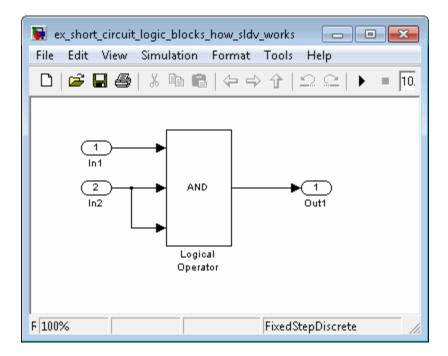
When the Simulink Design Verifier software analyzes this model for Condition Decision coverage, the analysis can only satisfy five of six objectives for the Logical Operator block inputs. The software cannot generate a test case when the third input to the Logical Operator block is false. If the second input is false, the third input is false, but the software ignores the third input due to the short-circuiting. If the second input is true, the third input is never false.
